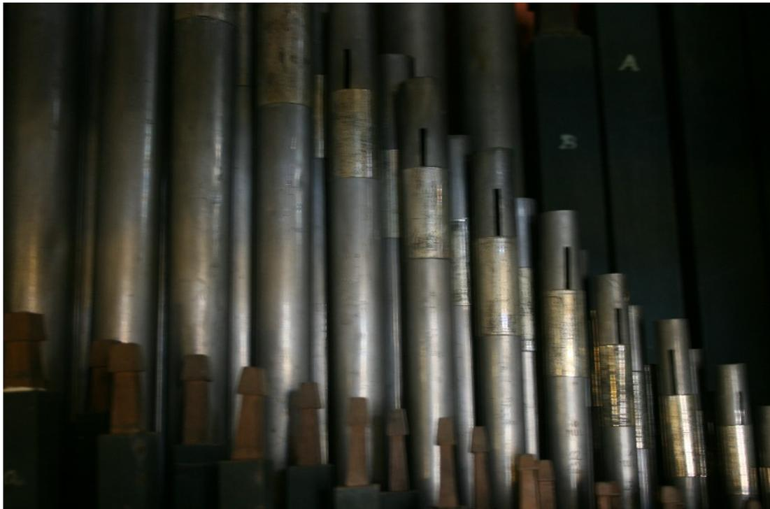
A new pedal chest will be made to enable all the pedal pipes to be placed behind the organ ensuring clean lines at the sides and giving the case a little further depth.
